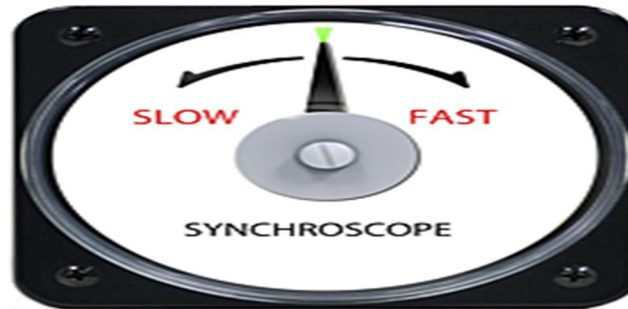
Figure 7 Synchroscope meter and synchronizing indicator
