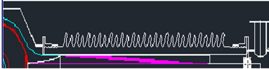
Figure 3: 2D view of 145kV live tank current transformer existing Capacitive graded bushing design
