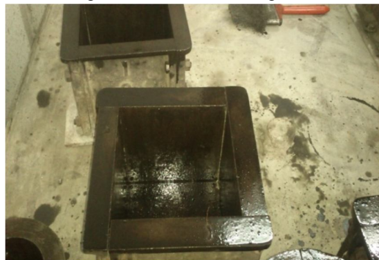
Fig 10: The cubes are being oiled
