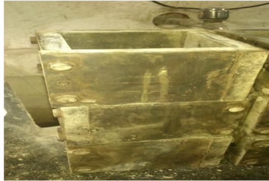
Fig 10: The cubes are being oiled
