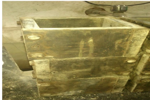
Fig 10: The cubes are being oiled
