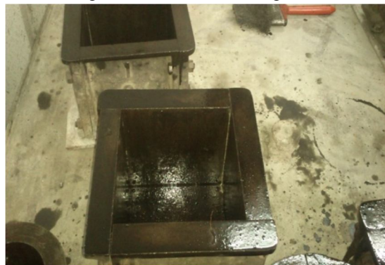
Fig 10: The cubes are being oiled
