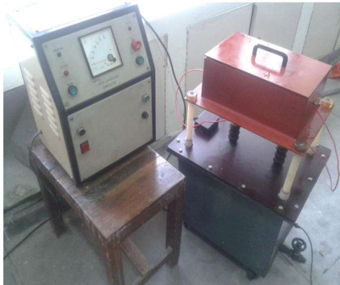
Fig-1: Solid insulation BDV experimental laboratory set-up.
