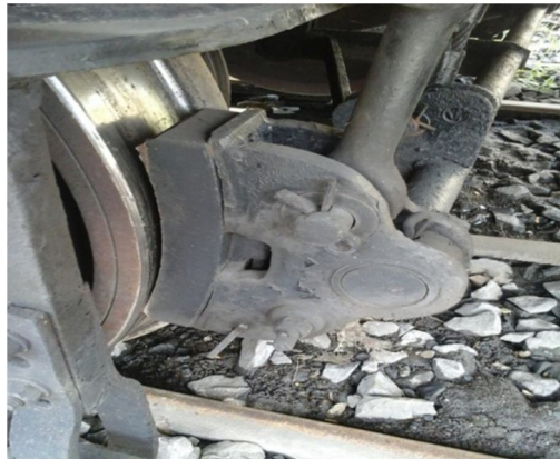
Fig1:-Brake shoe on ICF Bogies
