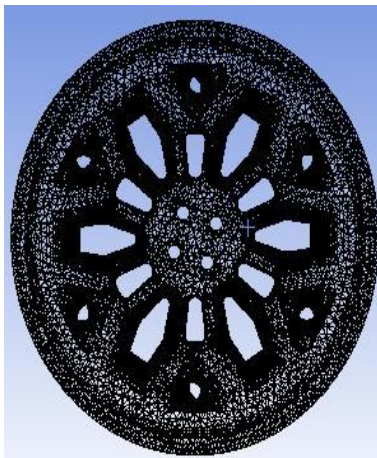
Fig. 4 Meshing of wheel rim
