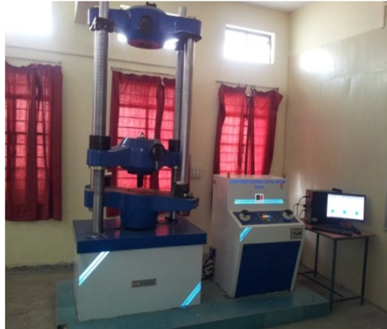
Fig. 1. Static test set up for both composite and steel leaf spring.
