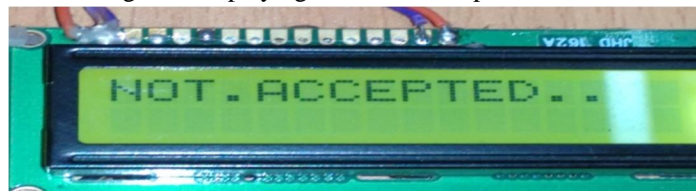
Fig :7.3 Displaying that unauthorized person try to open the door
