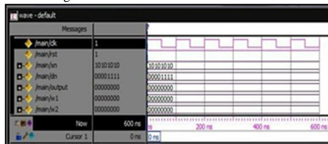
Fig.8. Simulation model of conventional DLMS adaptive filter for delay with X_n=10101010 , D_n=00001111 , R_{st}=1 And Clk=1
