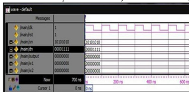
Fig.9. Simulation model of modified DLMS adaptive filter for delay with X_n=10101010 , D_n=00001111 , R_{st}=1 And Clk=1
