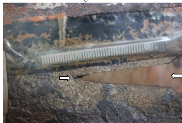
(d). 1,97,962 cycles Crack length: 39.77 mm
