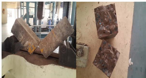
Fig 7. Testing of Beams
