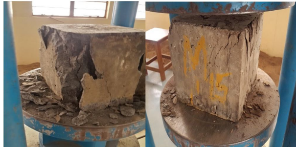
Fig 3. Testing of Cubes
