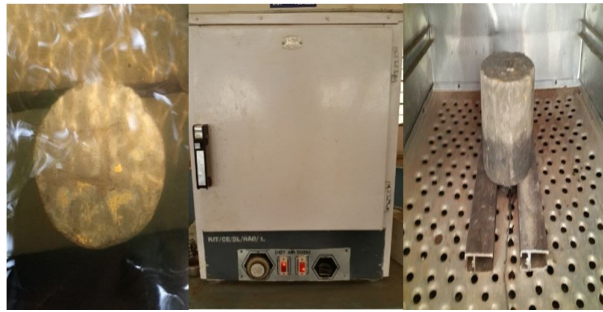
Fig 11. Curing and Hot air oven
