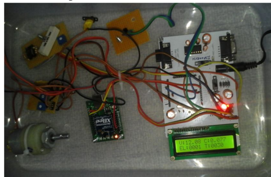
Figure2.2: Hardware used for Designing battery monitoring system
