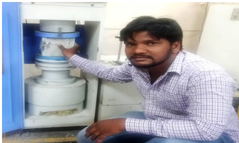
Fig. 1 testing of geopolymer concrete
