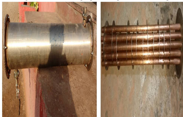
Fig.2: schematic view of Shell and Tube
