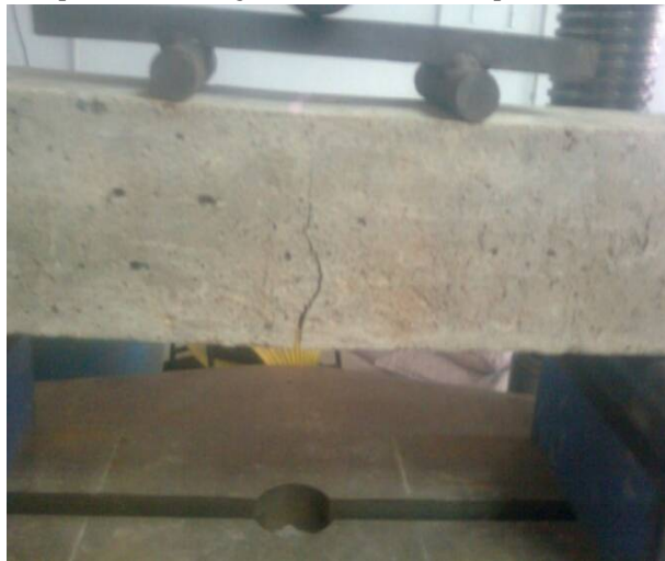
Fig 4: Testing of flexural strength test specimen
