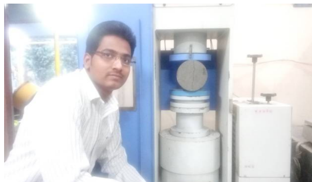
Fig -3: Testing of tensile strength test specimen
