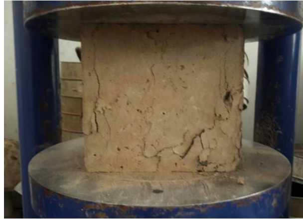
Fig 2: Testing of compressive strength test specimen
