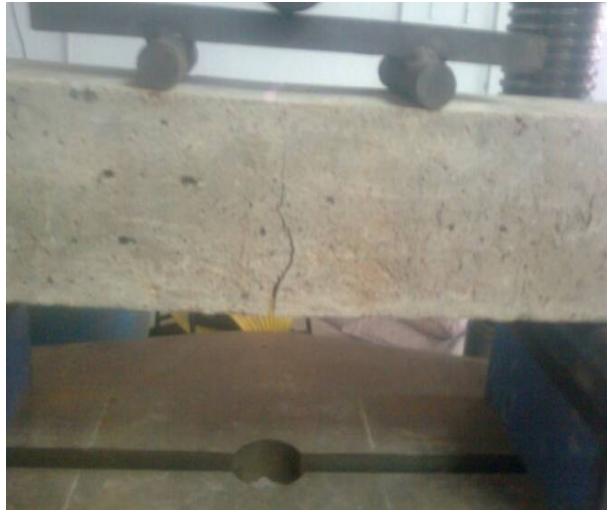
Fig 4: Testing of flexural strength test specimen
