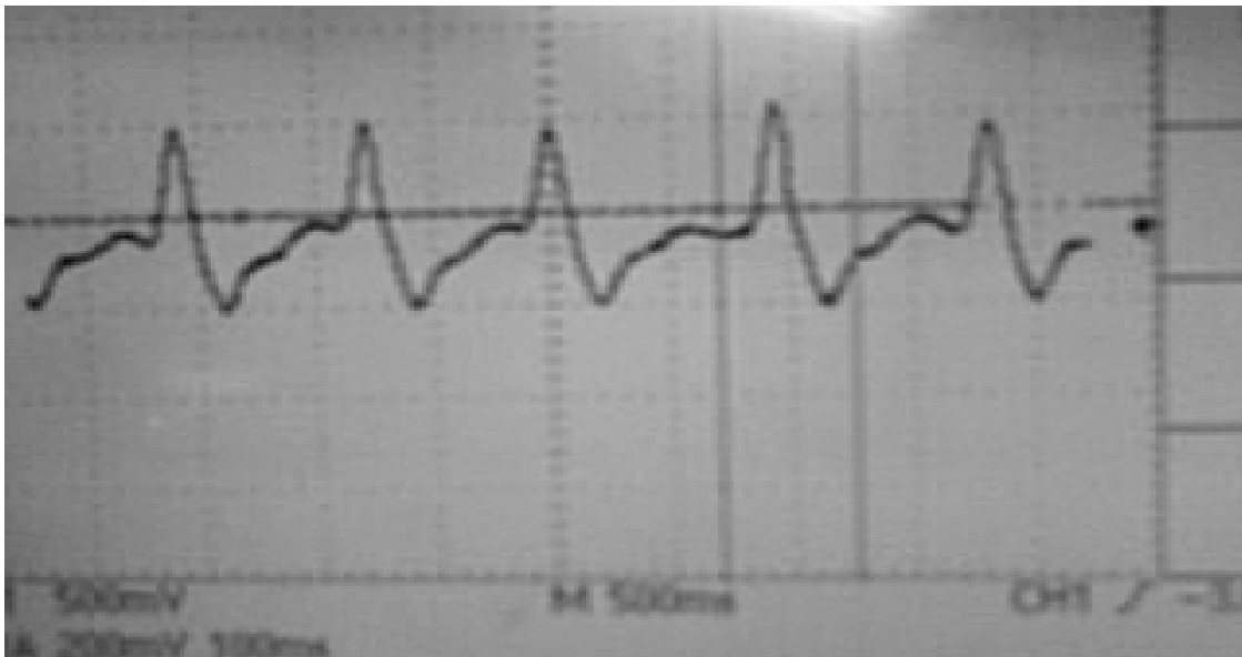
Fig. 3 Filtered output of 1 st stage BPF and amplifier
