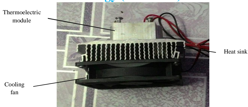
Fig. 3 Thermoelectric module with Heat sink and Cooling fan
