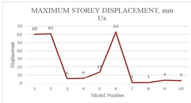
Fig. 2 Graph representing the maximum storey displacement in X direction
