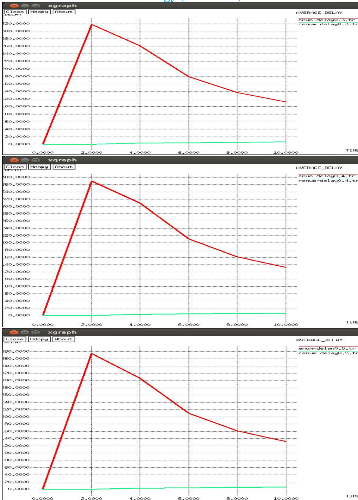
Fig 6 (a) Average Delay Lossless ENUM vs RENUM 0.3; (b) Average Delay Lossless ENUM vs RENUM 0.4; (c)
