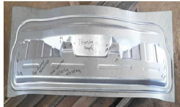
Fig.6 Actual component formed after tryout
