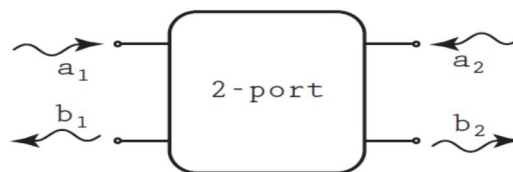
Fig.6. A two port with incident wave's a1 & a2 and reflected waves b1 & b2
