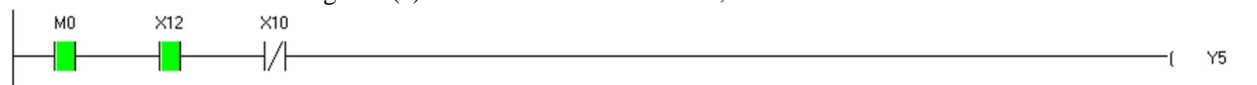
Figure 6(c): soil moisture sensor is ON but low water level sensor (Tank) is ON, so solenoid valve is OFF
