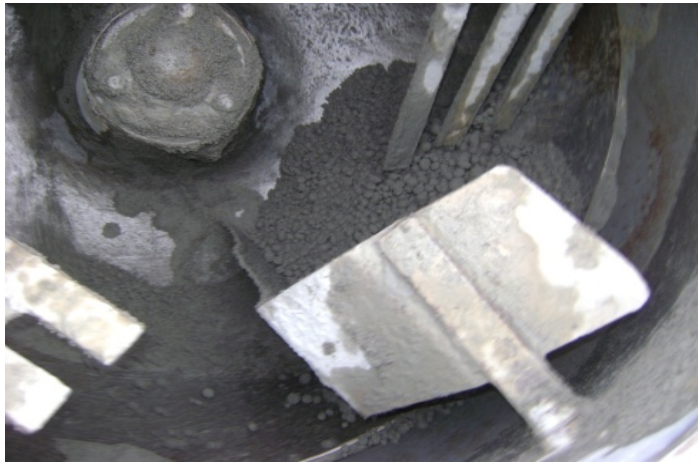
Figure 1 Formations of fly ash aggregates
