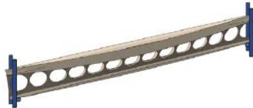
Fig 2. Lateral torsional buckling mode of cellular beams
