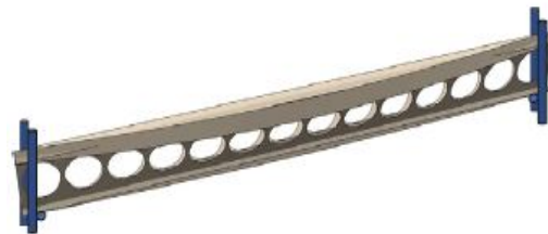
Fig 2. Lateral torsional buckling mode of cellular beams
