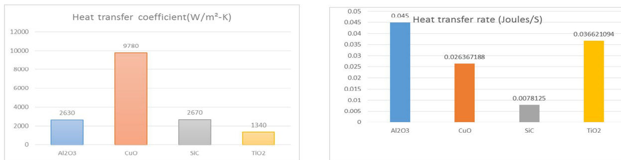
Fig. 12 Comparison of Heat Transfer Coefficient Values for All Nano Fluids
