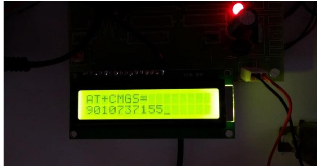
Fig: Mobile number that showing on LCD when accident occurs
