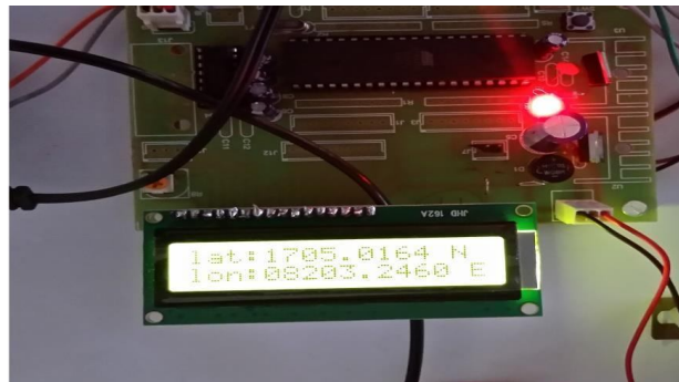
Fig: the latitude and longitude values of accident location given by GPS shown in LCD display.
