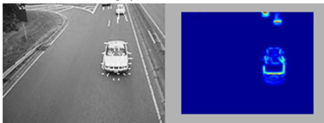
Figure 2: Optical flow estimation to obtain motion vectors (left) and pixel velocity magnitudes (right).
