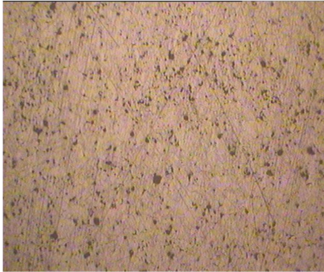
Figure 4 Optical Micrographs of Al - 2 wt. % Nano Al 2 O 3 Composite after sintering
