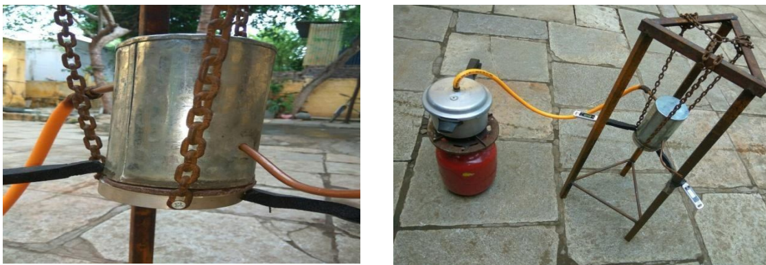
Fig. 2 Lee's Disc Apparatus
