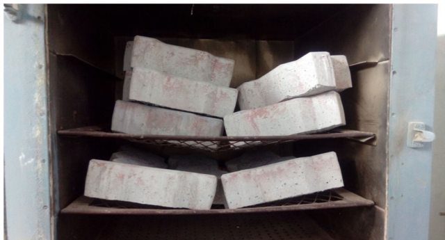
Paver blocks in oven
