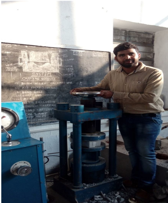
Compressive strength of paver block
