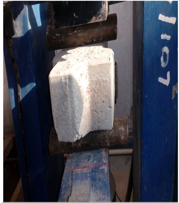
Flexural strength of paver block
