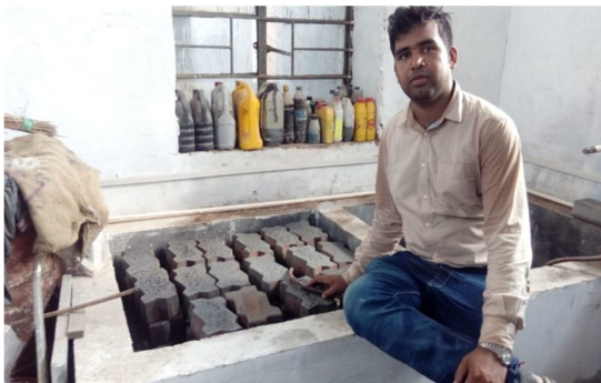
Curing of paver block
