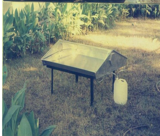
Fig.2 Double slope solar still
