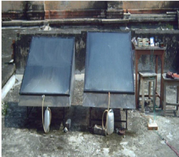
Fig.7 photograph of the conventional solar still and solar still with (right) and without PCM (left).
