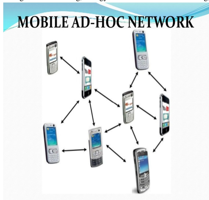
Fig.1 A Mobile Ad-Hoc Network (MANET)
