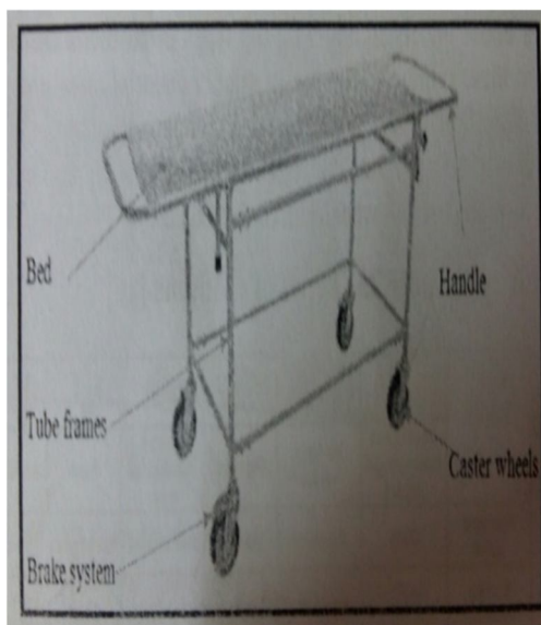
Fig. 1 Basic structure of stretcher
