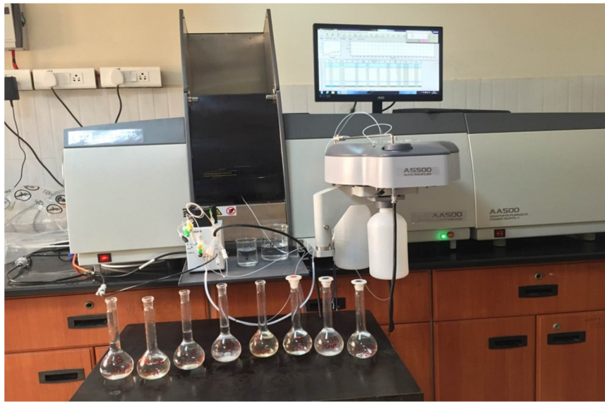
Fig 2.4: AAS instruments(AAS= Atomic Absorption Spectrophotometer)
