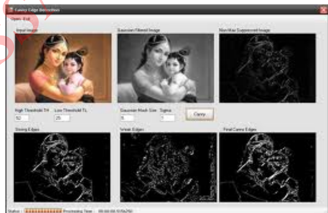
Fig.1.8. a) Original Image b) Smoothed image c) Non maxima suppressed image d) Strong edges e) Weak edge f) Final image
