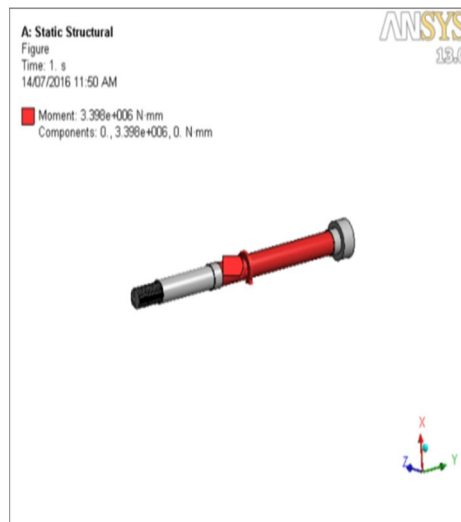
Fig:7. Moment applied on shaft
