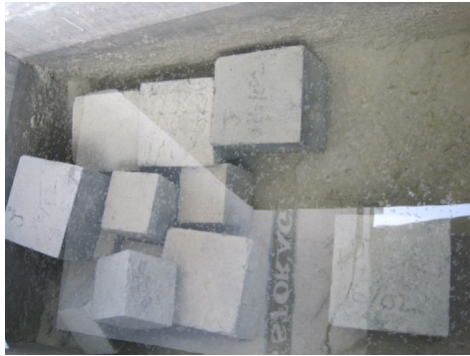
Figure. 1 Curing of Concrete Cubes (Mix+Nano-carbon Fibre)
