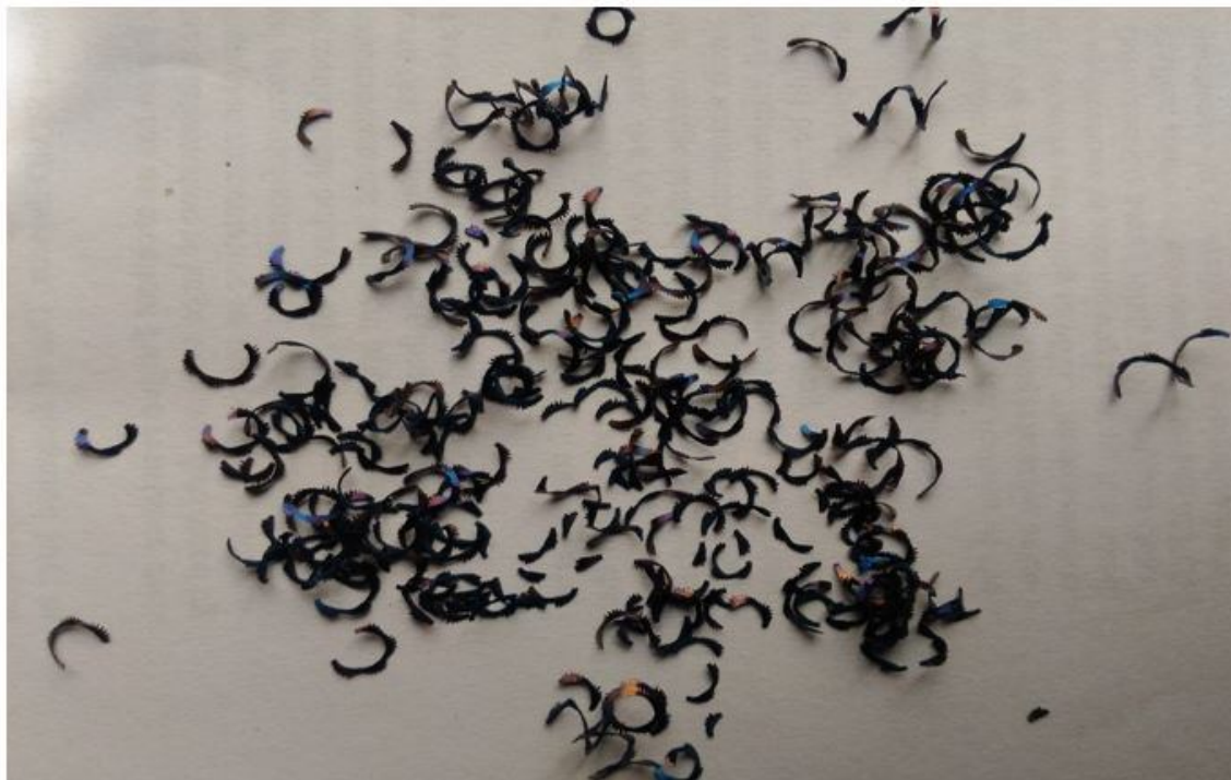
Fig 16: Discontinuous chips for DCT tool inserts
