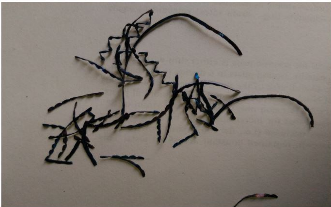
Fig 15: Partially continuous chips for SCT tool inserts
