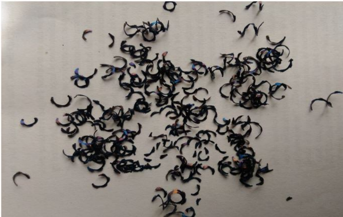
Fig 16: Discontinuous chips for DCT tool inserts
