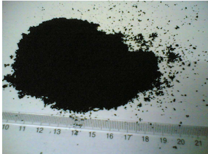
Fig 1. Crumb Rubber Sample
