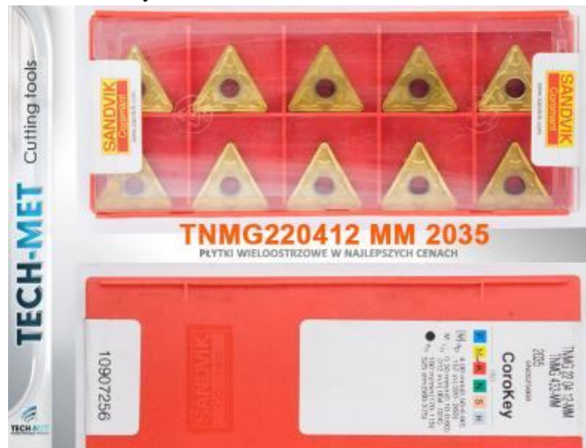
Fig.5 TNMG2204 tool used in this study
