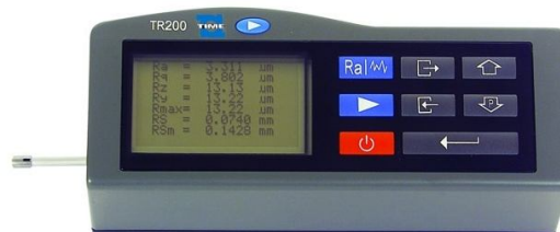
Fig.2 TR200 Surface Roughness Tester
