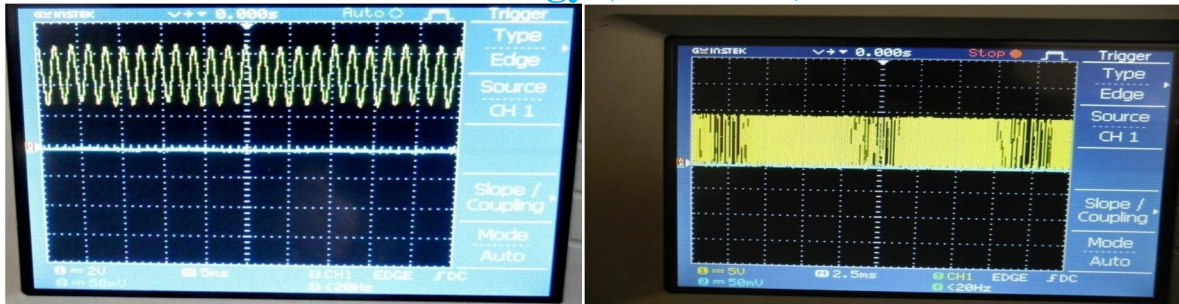
Figure 11: Output of amplifier for transmitter with Input Audio Signal 150Hz & Output of transmitter's VCO with Audio Signal 100Hz
