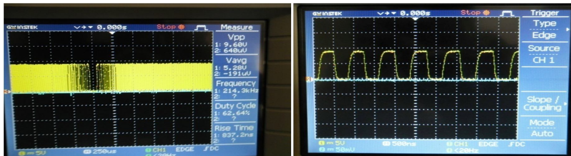
Figure 12: Output of transmitter's VCO with Audio Signal 200Hz, Output of transmitter's VCO with Audio Signal 10 kHz & Output of transmitter's VCO with Audio Signal 1 kHz
