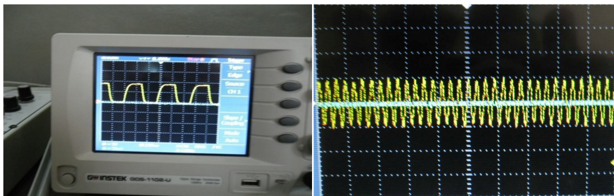
Figure 10: VCO output and the center frequency & Output of amplifier for transmitter with Input Audio Signal 50Hz
