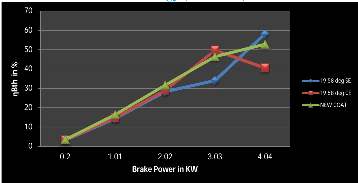
Figure 23: Brake power Vs Brake thermal efficiency.
