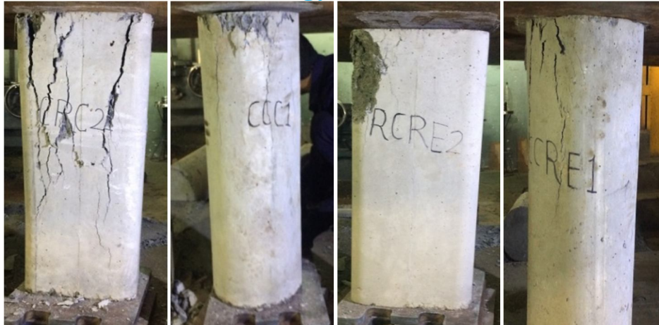
Fig. 9: Failure of Control Specimen and FECC
