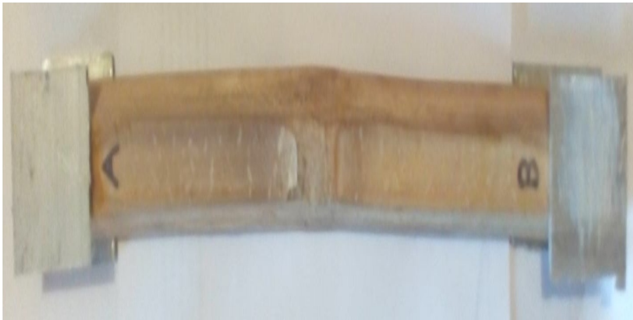
Fig. 5 Tensile Specimens with Aluminum Tabs
