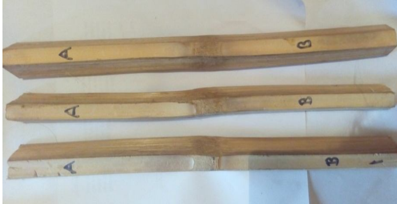
Fig. 1 Tensile Specimen without end grips
