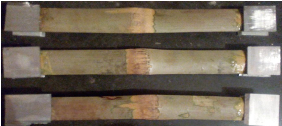
Fig. 6 Final Bamboo Specimens for tensile test
