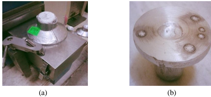
Fig. 3(a) Specimen of A356.0 on Spectro Meter and (b) Specimen of A356.0 for Chemical Composition Test
