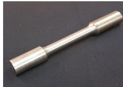
Fig.9 Tension Test Specimen
