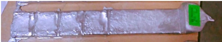
Fig.5 Specimen of A356.0 for Test of K-Mold
