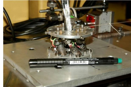
Figure 8: Force-torque sensor based on Gough-Stewart platform
