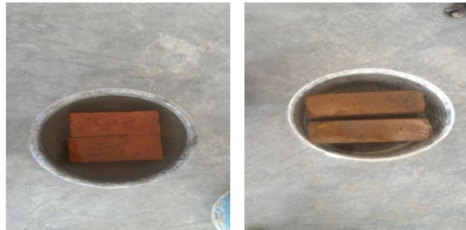
Fig.4 Water absorption test
