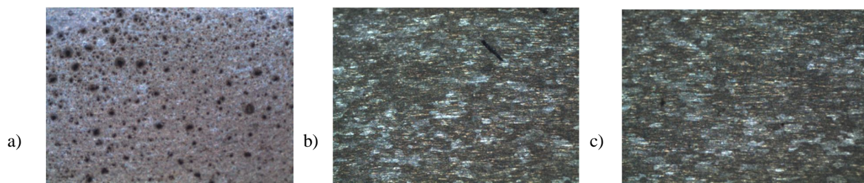
Fig.5 (a) Microstructure of cast matrix AA6061-T6/ Al 3 Fe, (b) after FSP 1 pass and (c) after FSP 2 pass
