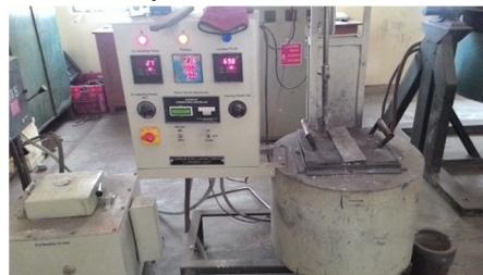
Fig; 1 Furnace used for In-Situ Fabrication of MMCs
