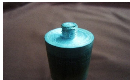
Fig; 2 Tool used for FSP
