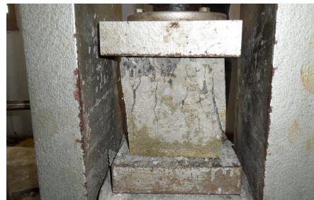
Fig 3 Failure mode (CWC 15%)
