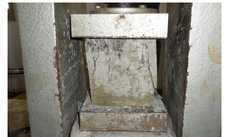
Fig 4 Failure mode (CWC 30%)
