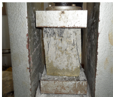
Fig 5 Failure mode (CWC 45%)
