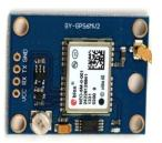
The NEO-6m series is a family of u-blox 6 positioning stand-alone GPS receivers featuring the high performance. The antenna is attached to the PCB with a little snap on coax connector. It can be carefully lifted off to disconnect. There are 4 connections, Tx,Rx,Vcc and Gnd.
